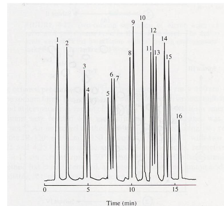
**FIGURE 4-29.** HPLC analysis of *o*-phthalaldehyde amino acids on a reversed-phase Microsorb Short-one C18 column (Rainin, Woburn, MA) using a 1.7 mL/min gradient elution of solvent A (0.1 M sodium acetate adjusted to pH 6.2 with acetic acid) and solvent B (methanol) with fluorescence detection. Peaks: 1 = Asp, 2 = Glu, 3 = Ser, 4 = His, 5 = Gly, 6 = Thr, 7 = Arg, 8 = Ala, 9 = Tyr, 10 = Abu, 11 = Met, 12 = Val, 13 = Phe, 14 = Ile, 15 = Leu, 16 = Lys.
